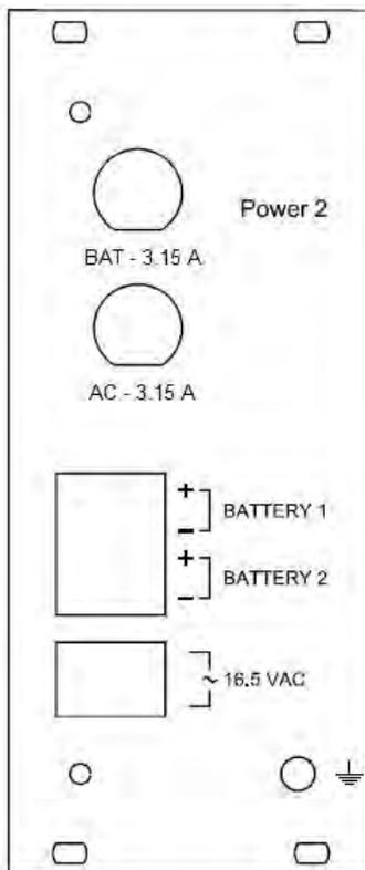
BAT – 3.15 A – Fuse to protect battery circuit.
