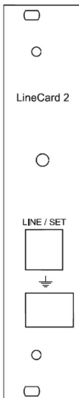
LINE / SET – Analog telephone line connector.
